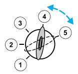
3. If the temperature is below  $-12^{\circ}$  C ( $10^{\circ}$  F) and the engine does not start in 15 seconds on the first try, turn the key OFF and wait 10 seconds and try again. If the engine does not start in two attempts, press the accelerator pedal all the way to floor and hold. Turn the key to START position.
